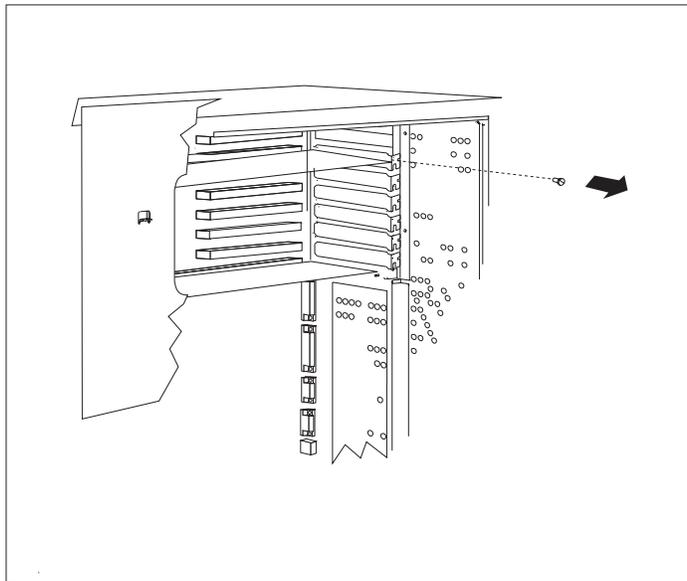
d. Carefully pull the adapter out of the system.
