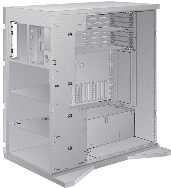
8. Slide the diskette drive and the CD-ROM drive forward in their guides to allow more room for connecting cables to the new drive.
