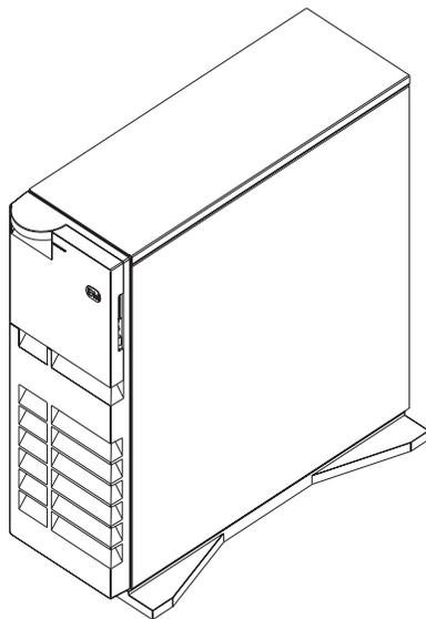
**Attention:** Be sure to maintain a clearance of at least 51 mm (2 inches) on all sides of the system to allow for air circulation.
