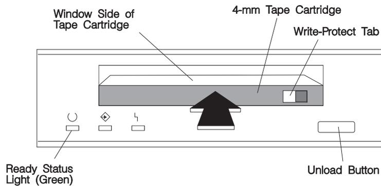
The 4-mm tape drive is ready for data operations when the tape cartridge is inserted. After the cartridge is inserted into the tape drive, the tape takes about 15 seconds to load.
