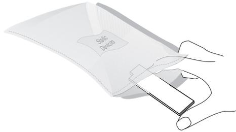
5. Replace the memory card, see “Installing or Adding Memory Adapter Cards” on page 5-20.
