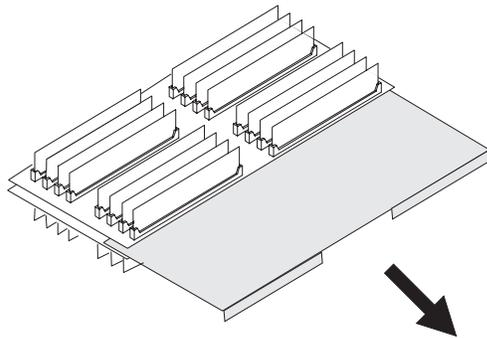
4. The card is secured in place with card retainer hooks, one on each end of the card. Open the card retainer hooks and remove the card.
