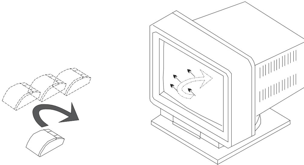
With the mouse buttons, you can perform functions such as selecting and deselecting options, extending your selection, or choosing a command. The precise function of your mouse depends on the software you are using.
