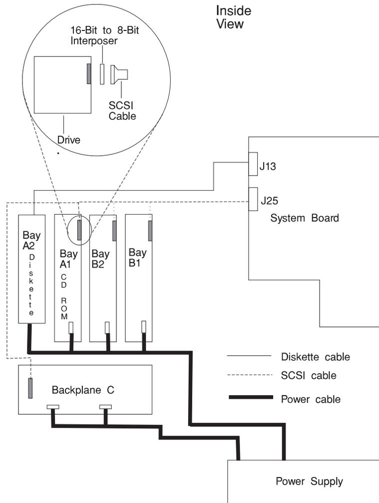
**Attention** Route the cables (SCSI-2 and power) at the rear of the media drives so they do not block airflow or bind between the fans and media drives.
