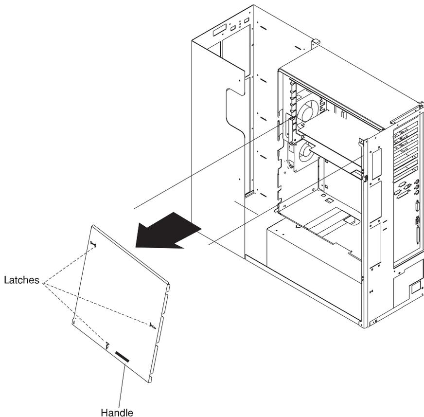
**Attention** If your system has the SSA bulkhead cable installed, make sure that you do not damage the cable as you remove the I/O planar cover.
