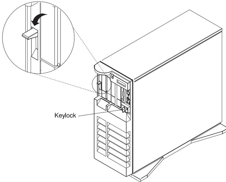
2. Reinstall the door at the front of the system by aligning the pins with the hinges, and sliding the door down.
