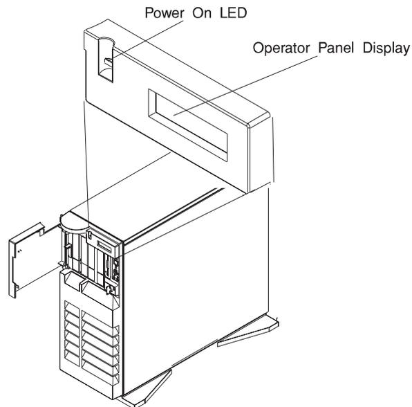
During power-on self-test (POST), 4 characters display indicating the progress of the testing. If an error is detected that requires attention, the system unit halts and an 8 digit number displays in the operator panel display to identify the error.
