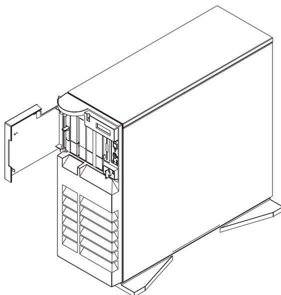
2. Remove the door by carefully lifting it up and off the hinges. Store it in a safe place.
