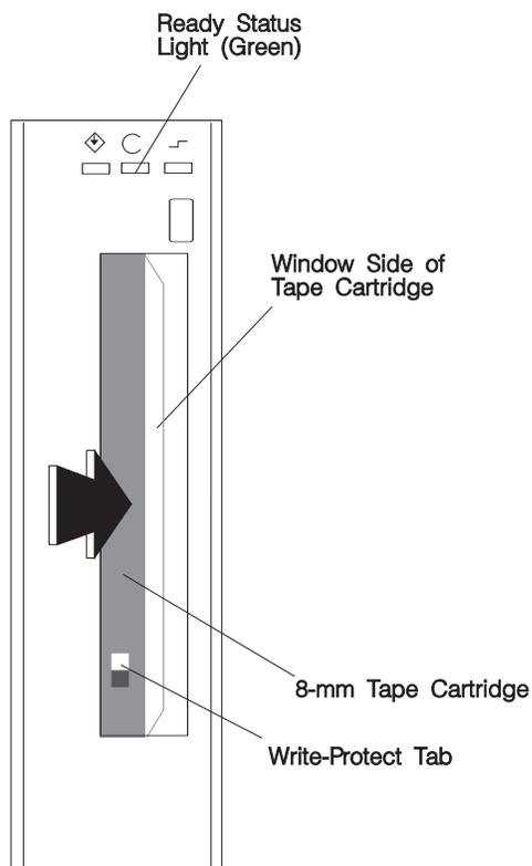
The 8-mm tape drive is ready for data operations when the tape cartridge is inserted. After the cartridge is inserted into the tape drive, the tape takes about 25 seconds to load; this does not interfere with beginning the data operations.
