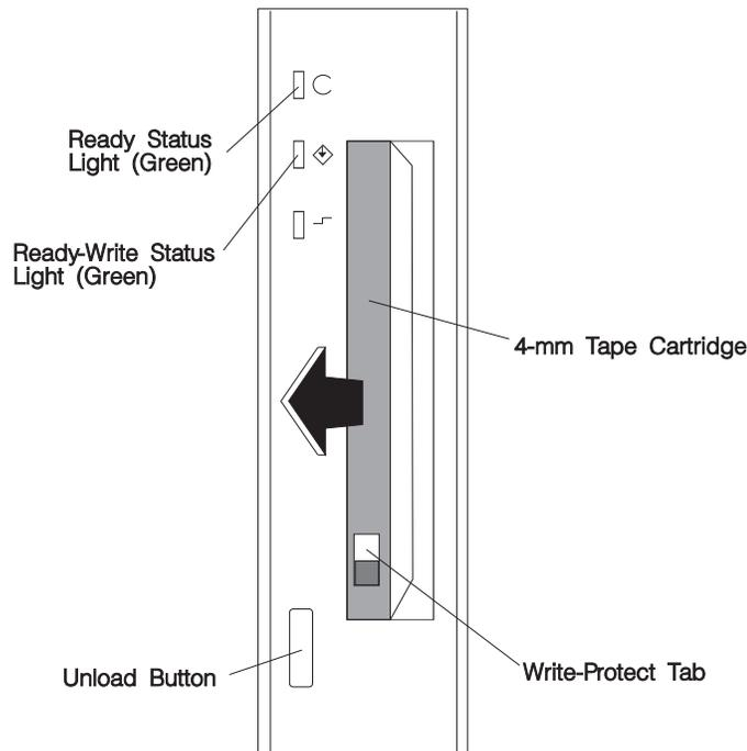
The time required for a tape to rewind and unload is between 10 seconds and 1.5 minutes, depending on the position of the tape when the unload button is pushed.
