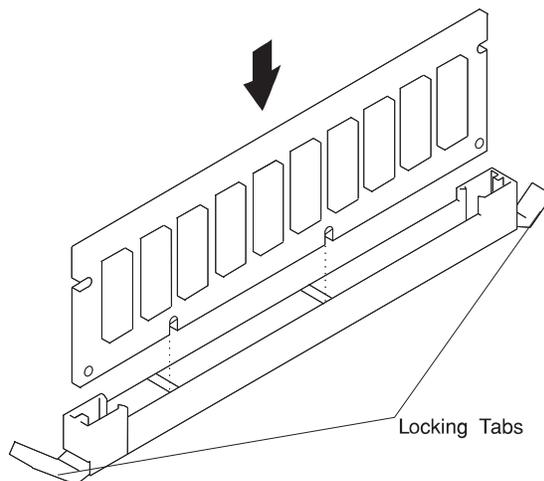
**Attention:** Inserting the memory-modules diagonally may damage the memory-modules.
