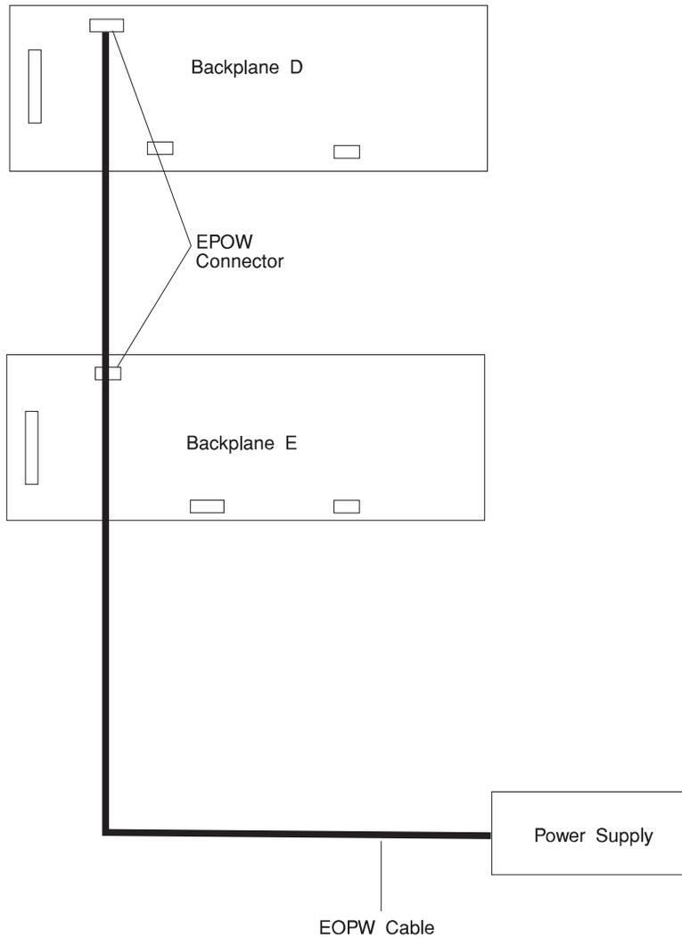
b. Attach the new power cable to backplane D or E.
