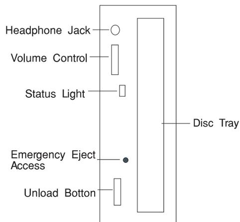
When the CD-ROM is set to On, the status light indicates one of several conditions. The following are status light states and the respective conditions of the CD-ROM drive:
