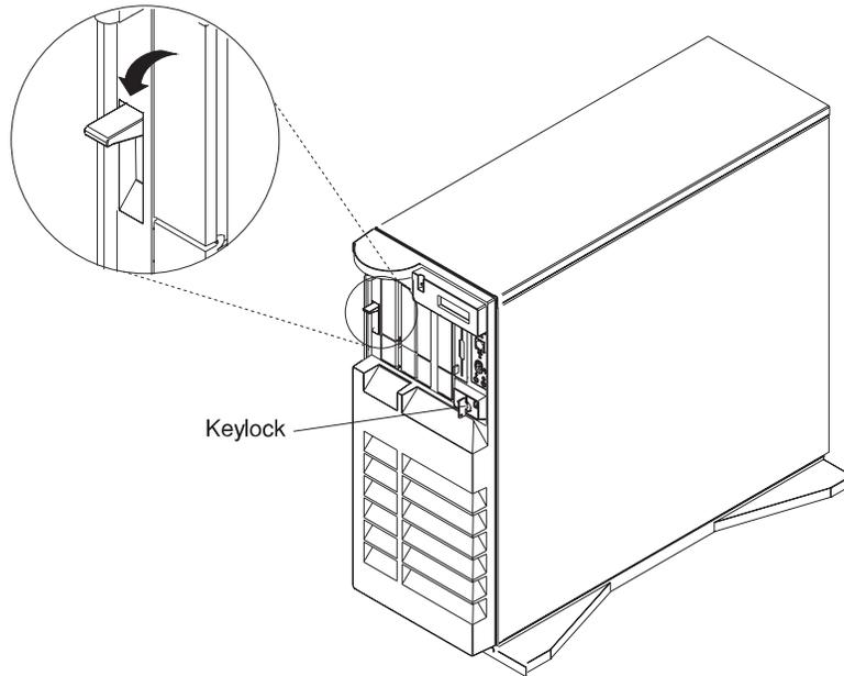
3. Reinstall the door at the front of the system by aligning the pins with the hinges, and sliding the door down.
