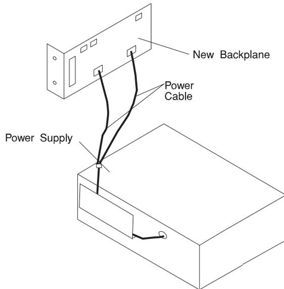
c. Connect the other end of the power cable to the power supply.
